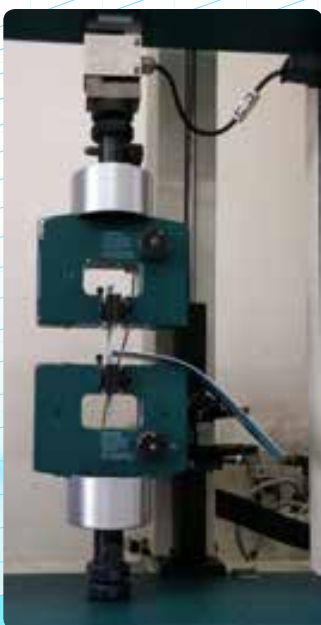
Peel Resistance Test in progress
